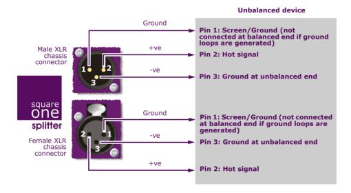
Figure 3: I/O connections to unbalanced devices
