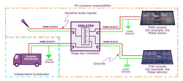
Isolated systems are the next step up from a passive system and offer a big increase in performance, although this comes at a price. To get the best out of an isolated system a very high quality transformer is required, which is expensive.
