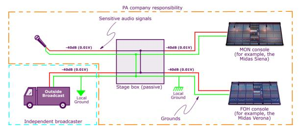
There are four fundamental problems inherent in a passive parallel type splitter:
