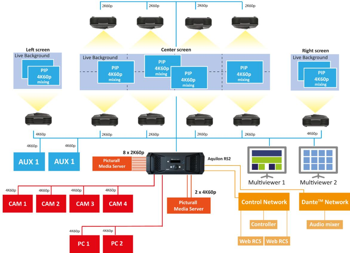
**Aquilon RS2 can drive 2x 8K60p LED walls and 4x 4K60p AUX outputs**
