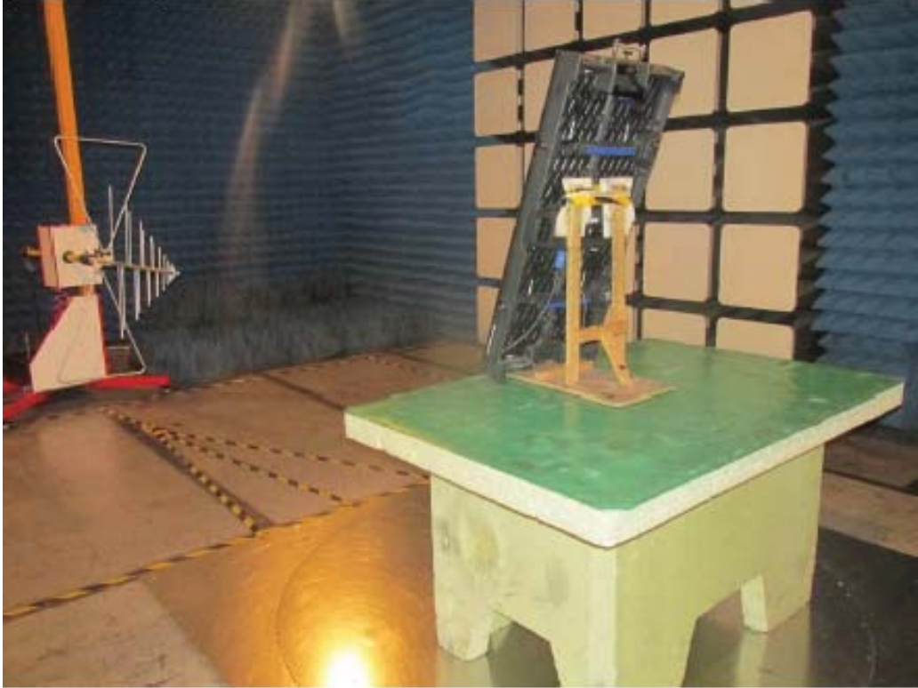
Photograph 3: Set-up for Radiated Disturbance
