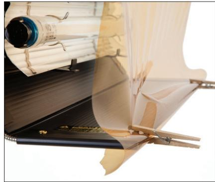
Restricting the airflow around the lamps can cause the lamps to operate hotter. This increased heat will raise the lamp's color temperature and green spike. Therefore, it is recommended to clip gels to the doors of the fixture.
