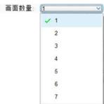
Take 2 (number of layers) as the example, select [Number of Layer] for 2, and the screen setup wizard will pop up. Select the input signal source of screen 1 in [Video Input], scale the screen 1 in [Screen Settings], click "I" to crop the screen 1, then click [Next] after completing.
