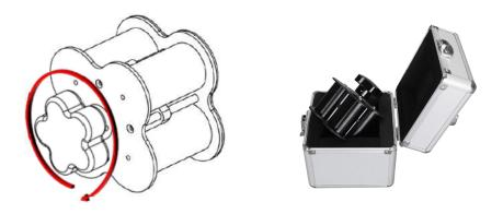
This magnet specially designed to carefully remove and replace the Qadra LED module from the front of the panel. Before using this tool, be sure that the magnet is drawn all the way back to the home position by turning the knob clockwise.
