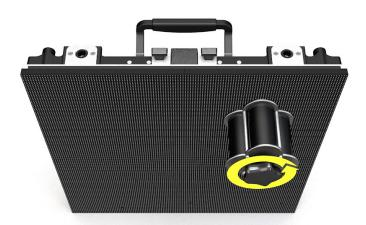
3. With steadily increasing force and as straight as possible, pull the extractor back until the module is released from the frame.
