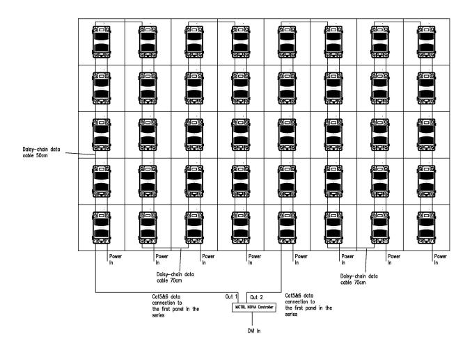
This solution is not using the redundancy data cable option. Connect power between the panels using the same procedure as the signal, only using the Power Input and Power Output connectors.
