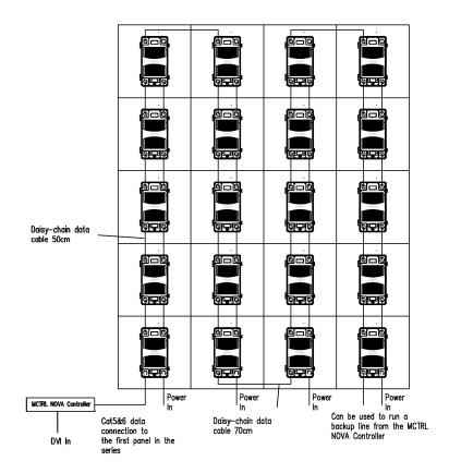
This diagram shows an example of a simple signal connection with backup data line for redundancy option.
