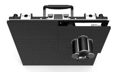
4. Release the module by turning the extractor knob clockwise.
