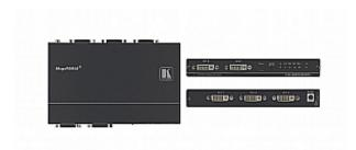
The VM-400HDCPxI is a 4K@60Hz (4:2:0) 1:4 distribution amplifier for HDMI signals via single-link DVI. It takes one DVI input, equalizes and reclocks the signal and distributes it to four identical outputs. With the appropriate adapter, it distributes signals having resolutions up to 4K@60Hz (4:2:0), WUXGA and 1080p.
