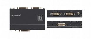
The VM-2HDCPxI is an HDCP compliant distribution amplifier for DVI-D signals with resolutions up to and including WUXGA and 1080p. It reclocks and equalizes the signal and distributes it to two identical outputs.
