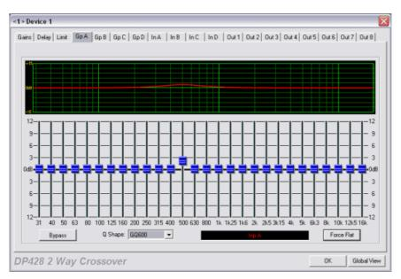
As can be seen by this example, the 500Hz band has been boosted by 2dB, and the bandwidth that has been affected is quite wide (there is still appreciable activity an octave on either side of 500Hz – 250Hz and 1kHz).
