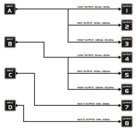
$2 \times 4$  way crossover: Inputs A and B feed four outputs each, with inputs C & D being unused. Default suggested crossover frequencies are shown by each output.
