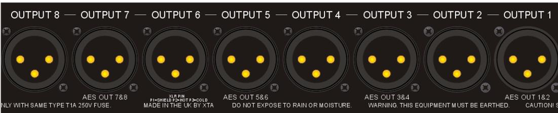
**Audio Outputs:** 3 pin XLR sockets are provided for each channel. All are fully balanced, pin 2 hot, 3 cold, 1 screen. Note the legending on the panel to designate which outputs are used for AES streams when the digital outputs are enabled. Please see page 33 for more information.
