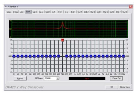
When the band is boosted to its maximum value, it can be seen that the response has become quite narrow. This is useful when cutting bands (for example to remove troublesome feedback resonances) as it has less effect on the surrounding areas.
