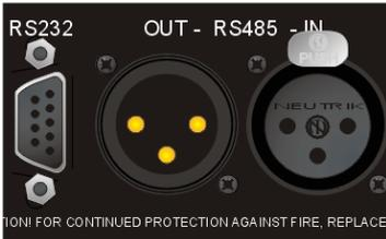
**RS232:** RS232 standard via a 9 pin D-type connector, for connection to a PC. Data is converted to RS485 standard and relayed to slave units via the RS485 sockets.
