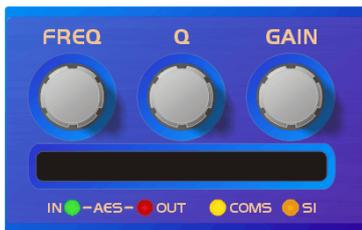
**Rotary Encoders:** Three velocity sensitive encoders adjust the relevant parameters as displayed on the screen.
