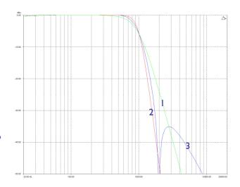
To produce a crossover filter of this shape it is simply a case of setting the low (or high) pass filter for that output to the desired crossover frequency, and selecting a 12dB Butterworth response:
