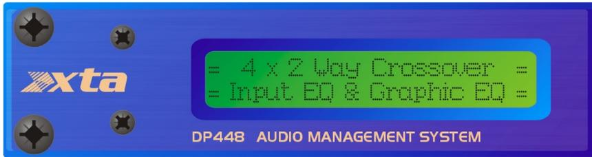
**LCD Screen:** Shows, by default, the name of the last recalled memory on the bottom line of the screen, and the current routing on the top line. Also used to show all parameters as they are edited, and all menu selections.
