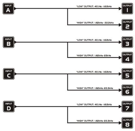
2 x 3 way crossover: Inputs A and B feed three outputs each, with output 7 being fed from input C, and output 8 from input D. Note the 'Aux' outputs are set to full range. Default suggested crossover frequencies are shown by each output.
