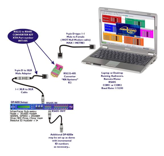
Both the converter and the required adapter cables are available from XTA. The adapter is available in a kit, which includes an RJ-45 adapter, the XLR to 9-pin adapter, and the converter itself. This complete kit is part number **INT-485**.
