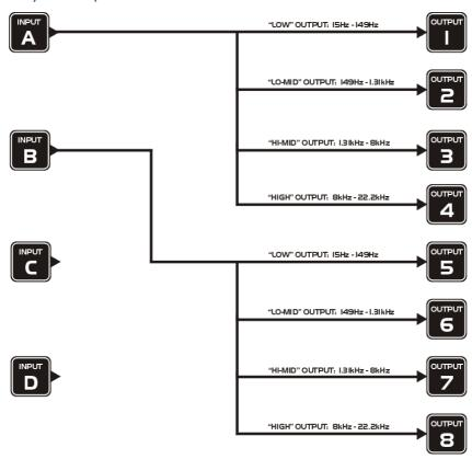
$\underline{I \times 8 \text{ way crossover}}$ : Inputs A is fed to all eight outputs, with initial settings being all full bandwidth. The crossover points can be adjusted as desired.
